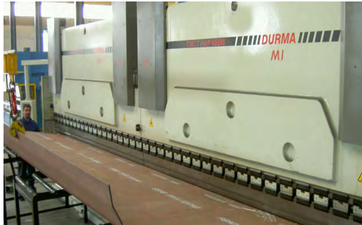
Bended wear-resistant steel plate. 8.000x2.500 mm. thickness: 10 mm. hardness: 450 brinell.
