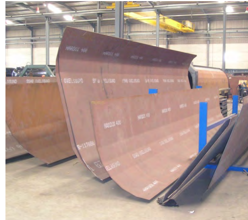
Bended plates ready for assembly
