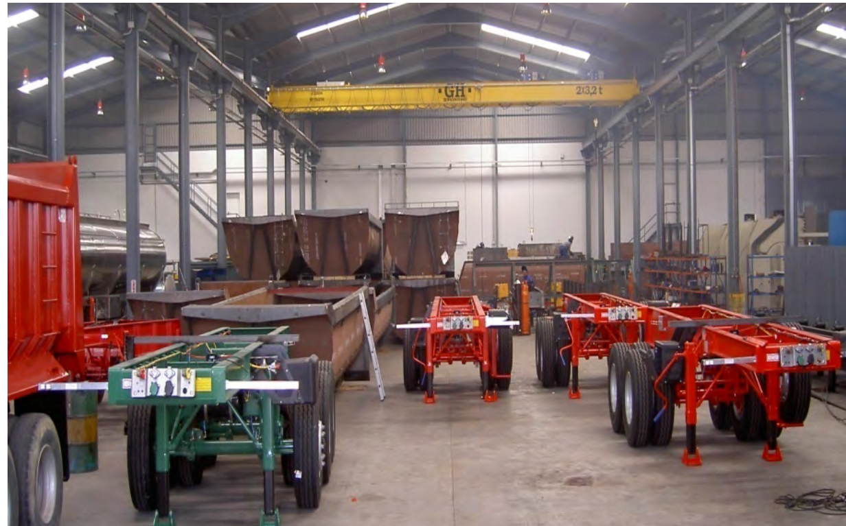
Assembly of tipper bodies on chassis.
