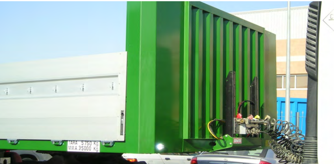
Plane front-end of 1.800 mm height.
